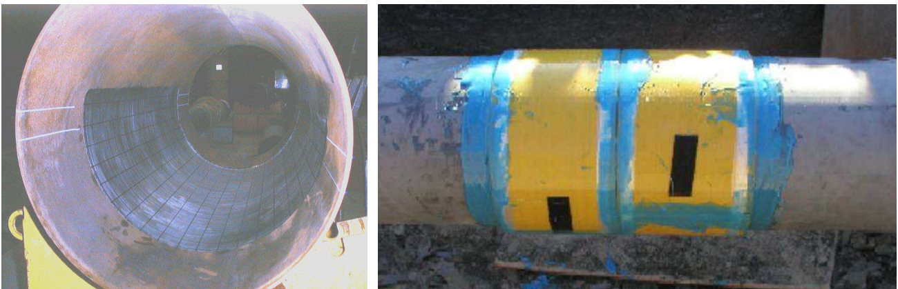
Figure 3 : Internal metal loss and Clock Spring
