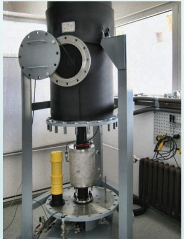
Figure 1: DBI test bench with controlled space and casing according to EG 97/23
