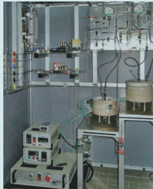
Figure 2: IFP test bench (2 permeation cells)
