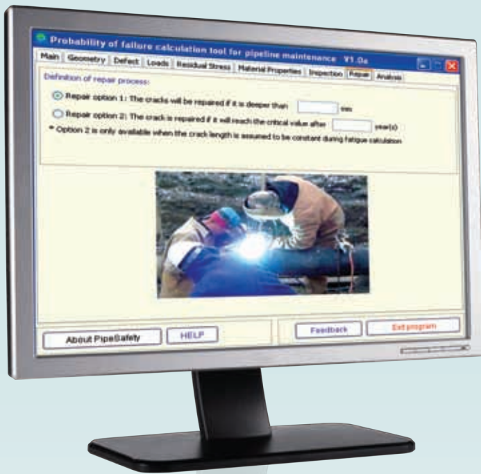
Figure 2: The pipeline management strategy also affect the probability of failure. Here the user can choose the repair policy on the pipeline
