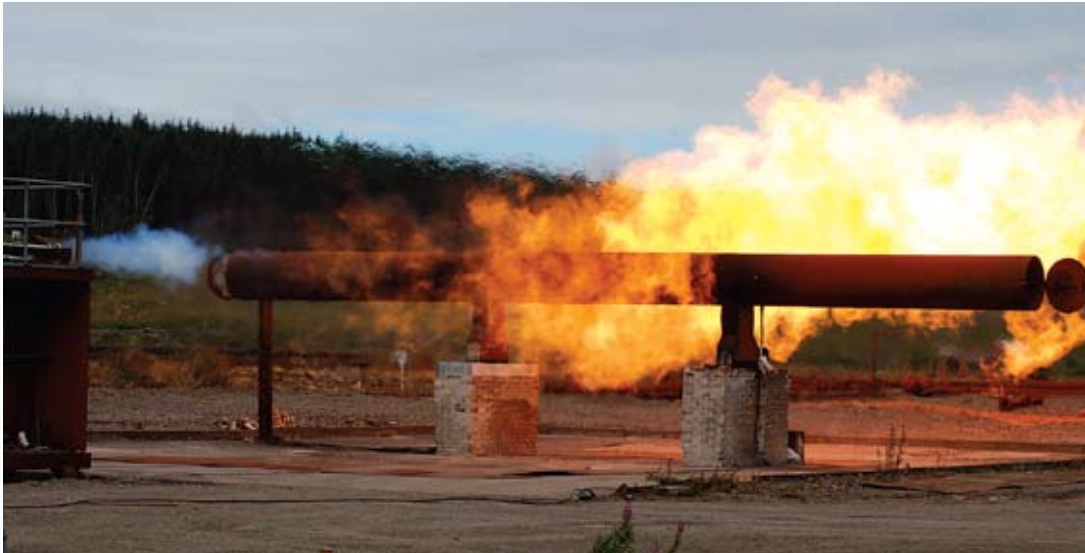
High pressure gas jet fire test at the Spadeadam test site
