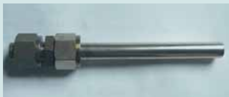
Figure 5: Pd thin film membrane supported on tubular ceramic substrate
